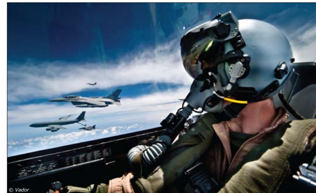
The aircraft banking away is carrying a pair of AIM-120B medium-range air-to-air missiles (stations 1 and 9), a pair of AIM-9M short-range air-to-air missiles (stations 2 and 8), a pair of GBU-12 500-lb laser-guided Paveway II bombs (stations 3 and 7), a pair of Sargent-Fletcher 370 US gallon underwing fuel tanks (stations 4 and 6), an AN/ALQ-131 ECM pod (station 5) and an AN/AAQ-33 PANTERA/Sniper XR targeting pod (station 5B).
