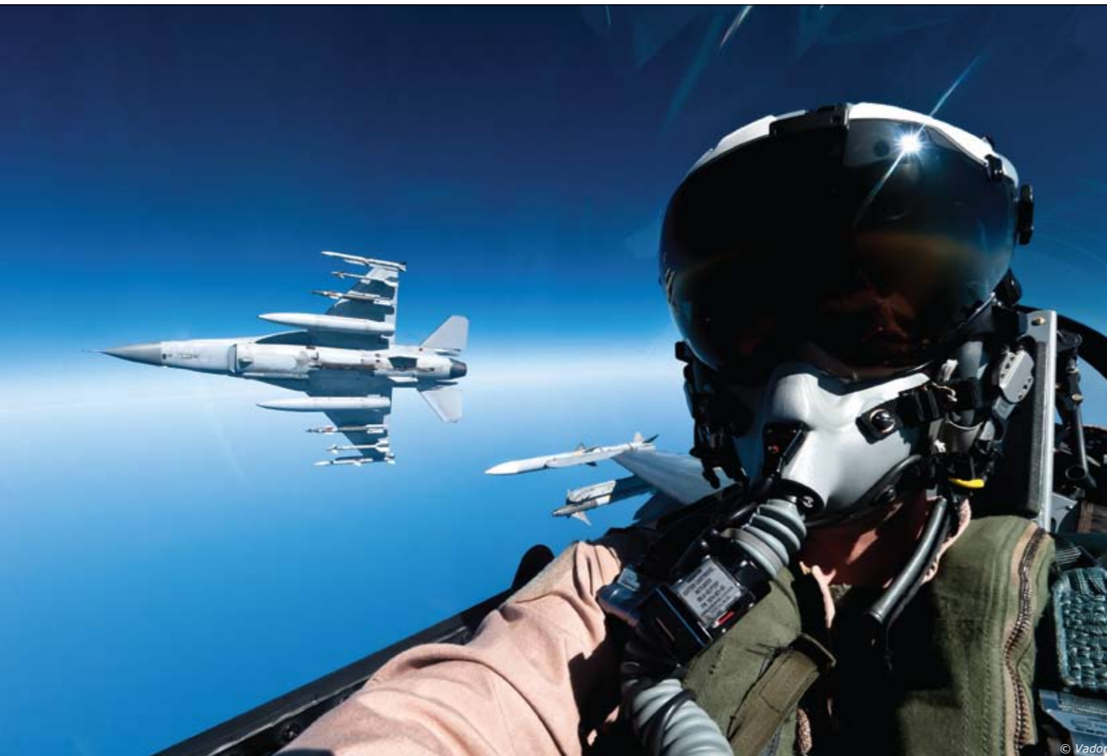
Left: Pilots participating in Operation "Freedom Falcon" wore a Video Systems International Joint Helmet Mounted Cueing System (JHMCS), but never used it to launch air-to-ground weapons because the sensors of the AN/AAQ-33 PANTERA/Sniper XR targeting pod offered much more precision for this purpose.
